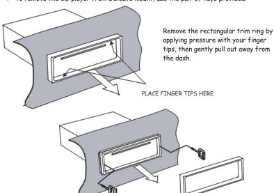
Insert the provided removal key into the opening on each side of the CD player. Push the keys inward until they snap in place. Firmly grab the keys and slowly pull the CD player out away from the dash.
